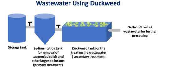
*Figure 3. Schematic diagram illustrating the stages involved in the treatment of the wastewater by the utilization of the duckweed( designed by author after [43].*
